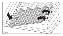
■ To take out the grease filters, release the locking clip on the filters, lower the filters 45°, unhook them at the back and remove them
